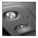
If your vehicle has reading lamps, press the button located next to the lamp to turn it on or off. The lamps can be adjusted to point in the direction you want.
